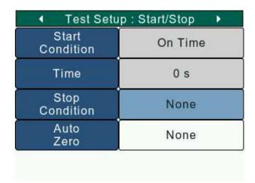
If the Stop condition is set to 'On Time', the user gets to set the test duration. The stop timer is visible on the Home (HomeScreen.html) screen indicating the time left in seconds. The user can enter a value between 0 - 3600 s as the stop duration.
