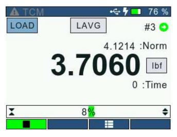
This load averaging test allows you to set a pre-load limit value or load threshold. The Preload value represents the "Start" and "End" point for your averaging function. The gauge will begin to collect and average the measured values once the "Preload Value" has been reached. The gauge will continue to average until the measured load drops below the Preload value. When the test is completed, the gauge will display the "Average Load".
