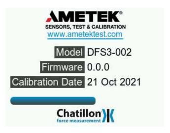
When the gauge is powered on, the Splash screen is displayed for approximately 5 seconds. This display shows AMETEK STC and Chatillon® logos along with Gauge Model, Firmware Version and the Last Calibration Date.
