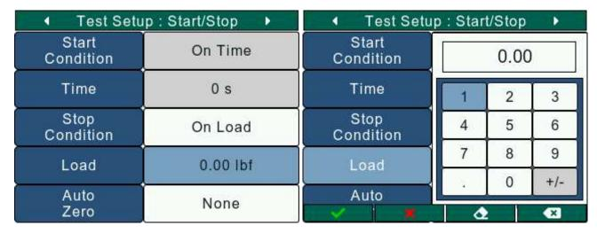
Stop Condition 'After Averaging' is available only if Load Averaging is enabled in Test Setup: Configure (TestSetupConfig.html) screen. In this case, the test stops once load averaging is completed.
