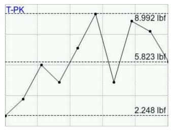
The F4 button can be pressed by the user to get a plot for the current result. The DF3 Series gauge allows the user to plot upto 300 data points and also displays Max, Min and Mean plotlines. If limits are on for the result selected, the user will also be able to see the high and low limits set by the user.
