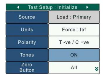
If the Tones setting is ON, the buzzer will notify to the user a Load Limit is reached.
