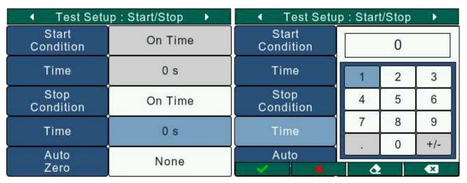
If the Stop condition is set to 'On Load', the user gets to set a load value, upon reaching which the test stops. The load value set by the user must be less than the maximum gauge capacity.
