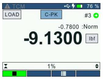
When the gauge is in Peak Compression mode (C-PK), the gauge will display the maximum compression load that was measured by the loadcell sensor. In addition to that, the user will also be able to view the Peak Compression value as a sub-reading when the gauge is in Normal or Compression Break (C-Brk)
