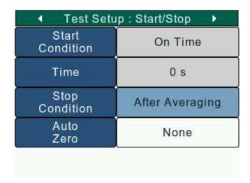
Stop Condition 'On Break' is available only if Break Detection is enabled in Test Setup: Configure (TestSetupConfig.html) screen. This option is available only in the DFS Series gauges. In this case, the test stops once break is detected.
