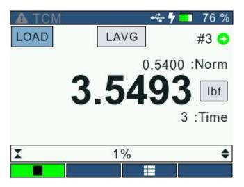
This load averaging test works identical to the Force-Based method except it adds "Time" as a factor. You may set the Timeout Value from 1 second to 3600 seconds. The gauge will begin to collect and average the measured values once the "Preload Value" has been sensed. The gauge will continue to average until the measured load drops below the preload value OR until the specified time has elapsed. When the test is completed, the gauge will display the "Average Load".
