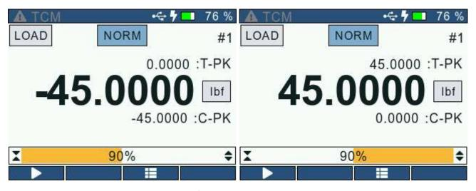
When the applied load is greater than **90%** of the maximum range, the load bar graph is **Red** in colour.
