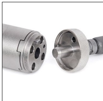
Fig. 10.1 The attachment and main sensor body mate with a pin and threaded ring.
