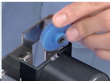
Replacing a gear
