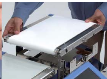
Replacing a conveyor
