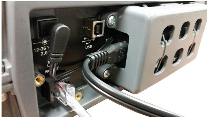
**Figure 2.5 AC power connections**
