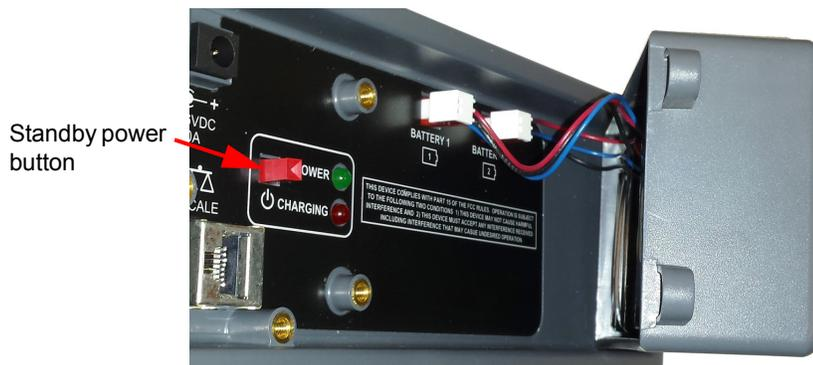
Figure 2.6 Battery pack connections
