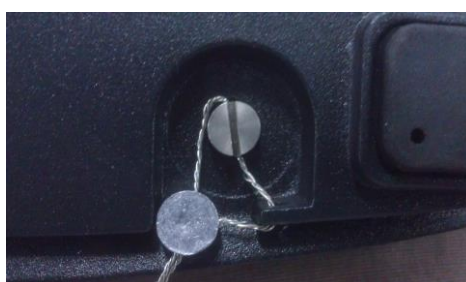
Locked with Wire Seal
