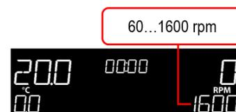
2. To turn on the stirrer, press and hold the right knob (D) until the unit beeps and the stirrer indicator (Q) illuminates.
