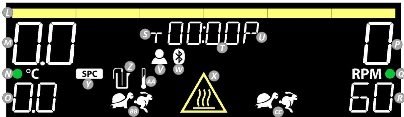
**L. Heater Indicator Bar:** Illuminates when the heater is  $\geq 40^{\circ}\text{C}$ .
