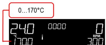
**Note:** While using the external probe, SmartHeat™ will still limit the temperature of the heater. This may cause the sample to heat at a slower rate and peak at a lower temperature than the SmartHeat™ setting.
