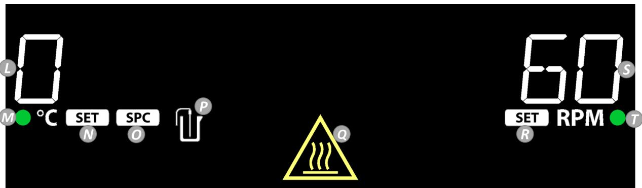
**L. Heater Temperature:** Switches to external probe temperature when the probe is plugged in and P is illuminated.
