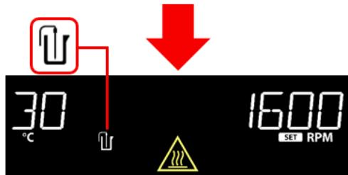
3. If the Ohaus External Temperature Probe is inserted into the external RTD probe port (E) while the heater is running:
