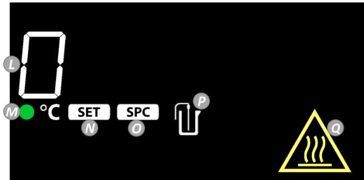
**L. Heater Temperature:** Switches to external probe temperature when the probe is plugged in and P is illuminated.
