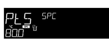
18. Press and hold the left knob (C) until the unit beeps to begin SPC at that temperature.
