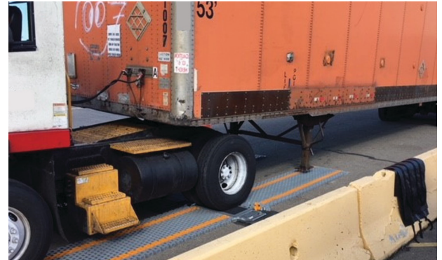
LS630-WIM™ Systems were chosen as an efficient method to screen incoming containers for proper gross weight to ensure safe transport.
