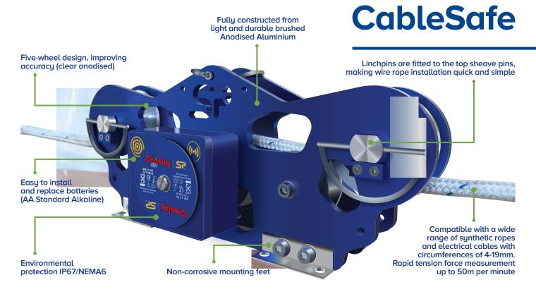
In addition to the TIMH range, the CableSafe is the continued evolution of Straightpoint's running line tensiometers. When used in the field, it will allow the user to monitor tension with exceedingly high levels of accuracy, which ensures rope/cables do not become overstretched or break.
