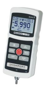
Thank you for purchasing a Mark-10 Series 5 digital force gauge, designed for tension and compression testing applications from 0.12 lb to 1,000 lb (0.5 N to 5,000 N) full scale. The Series 5 is an essential component of a force testing system, typically also comprising a test stand, grips, and data collection software.
