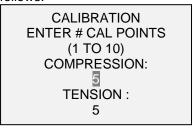
The gauge can be calibrated at up to 10 points in each direction. Enter the number of calibration points for each direction (compression and tension). At least one point must be selected for each direction.
