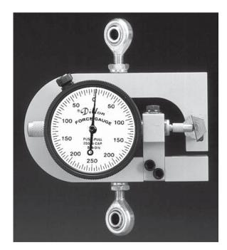
These bearings are available for all tensile models as standard equipment. They are a perfect fit and without any side play. Bearing pins can be machined from drill rod to suit your particular test plan. Remember that if you require a special adapter of some kind in place of these bearings, be sure that such adapters are self-aligning so that applied force is always able to assume a vertical line.
