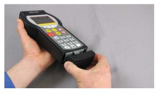
2. Press the tab of the gray battery box. The battery box will pop out slightly. Pull on the box to remove it from the Communicator.
