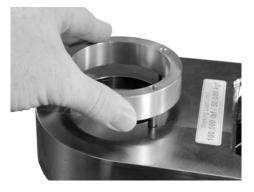
Figure 7.4 Placing Second Spacer on Roll Pins
