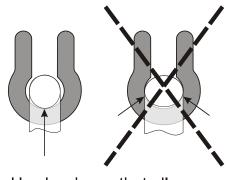
Use hardware that allows single point attachment and freedom of alignment. Do not use hardware that is undersize or restricts self-alignment. This results in poor measurement performance and possible dangerous safety conditions.
