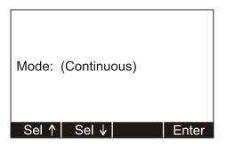
6. Select a mode of communication you want using the **Sel** keys to scroll through these choices; *Continuous*, *Poll*, *Remote* and *Print Key Only*. Press **Enter** to accept the setting.
