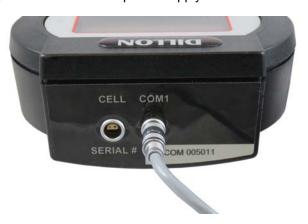
Figure 2.7 External Power Supply Connection (Communicator)
