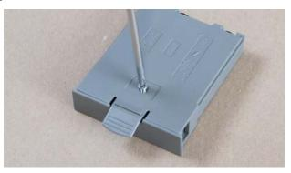
4. Remove the batteries (with a screwdriver if necessary) and replace with new AA batteries. Be sure to observe polarity when installing new batteries.
