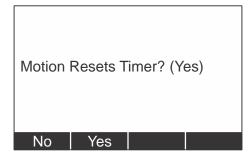
6. Select **Yes** if you only want the instrument to automatically shut down when there is inactivity. Select **No** if you want the instrument to power down after the timer counts down, regardless of any activity.
