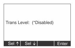
2. Select a transmission level using the **Sel** keys to enable as RS-232 or disable. Choices are; Disabled (default), RS232. Press **Enter** to accept the setting. See note below.
