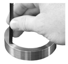
Figure 7.2 Inserting Roll Pin
