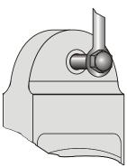
Use only the original factory equipment pins and shackles. Pin fit is critical and will affect accuracy.
