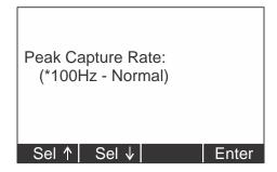
Select a Peak Capture Rate using the Sel key to scroll through the choices. Choices are 100Hz - Normal (default), 1kHz - High Speed, and 10Hz - Battery Saver. Press Enter to accept the displayed setting.
