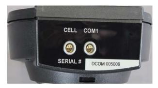
Figure 2.6 CELL and COM1 Connectors
