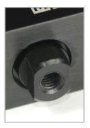
^ The load cell shaft includes flat surfaces as well as a threaded hole to accommodate attachments.
