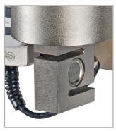
^ Series R01 sensor with shortened cable is shown mounted to an ESM1500LC test stand.\*
