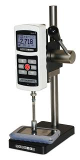
The ES05 is shown in a switch contact activation test, with Series 5 digital force gauge, extension rod and rubber tip attachment.
