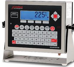
The calibration information is stored non-volatilely on both the main board and the digital load cell card in the 225D weight indicator. In the event of damage to either board, once replaced, the 225D will recognize the new board and automatically write the calibration data to the replaced board. Downtime is kept to a minimum since the indicator does not need to be recalibrated to the scale.
